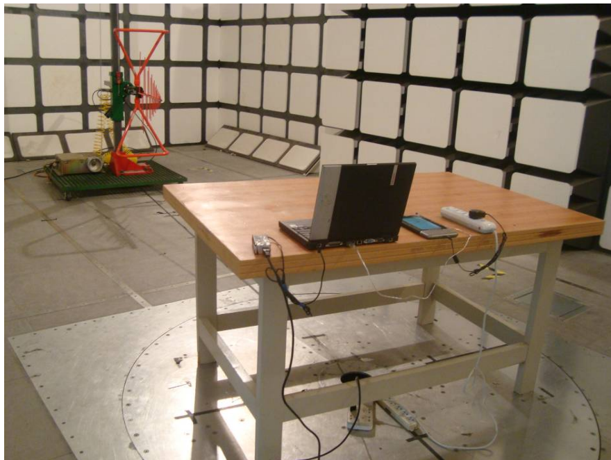
Below 1 GHz: Spurious Radiated Emissions - Rear View
