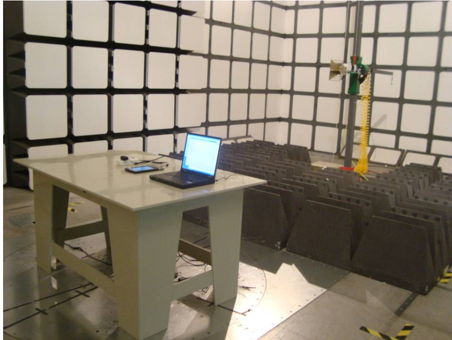
Above 1 GHz: Spurious Radiated Emissions - Rear View
