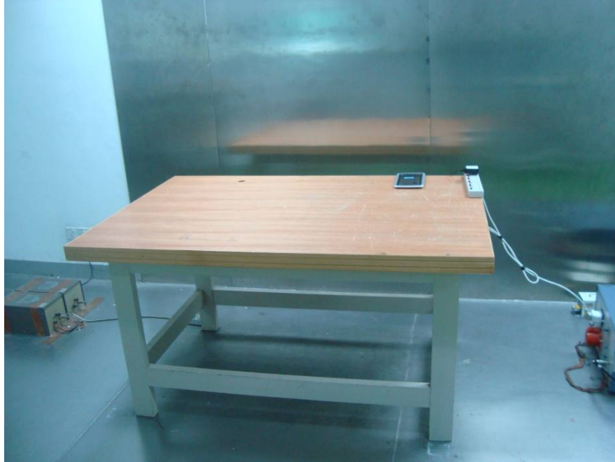
AC Line Conducted Emissions - Side View
