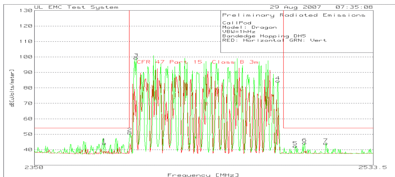
Band Edge Data with reduced VBW (1kHz) to simulate average measurement
