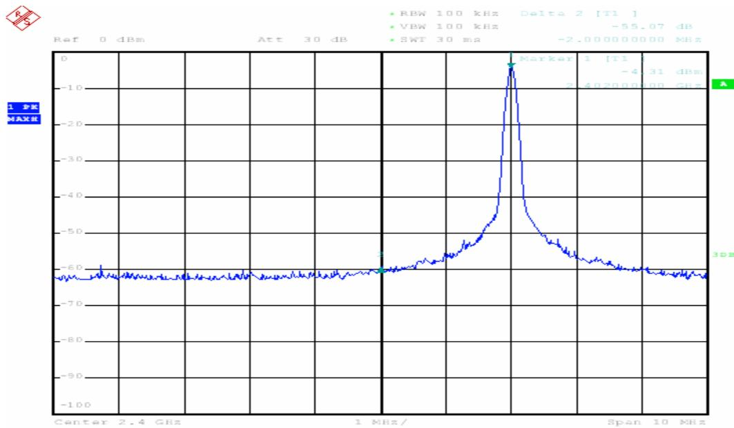
2. For highest Channel: the fundamental frequency is **2.4835G Hz**.
