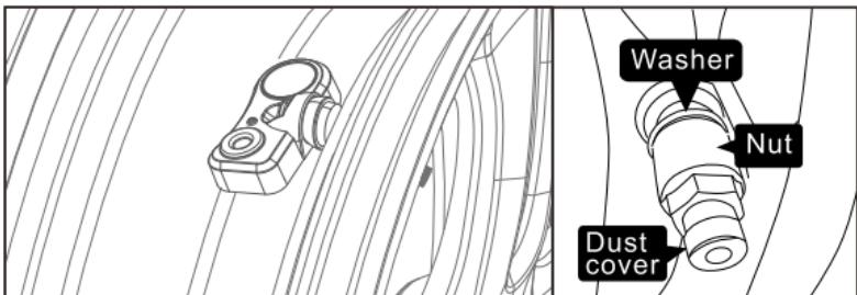
Step 5. Re-screw back the washer, nut & dust cover, load tire to vehicle and inflate.
