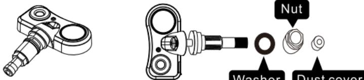
Step 2. Screw off the dust cover, nut & washer from sensor.
