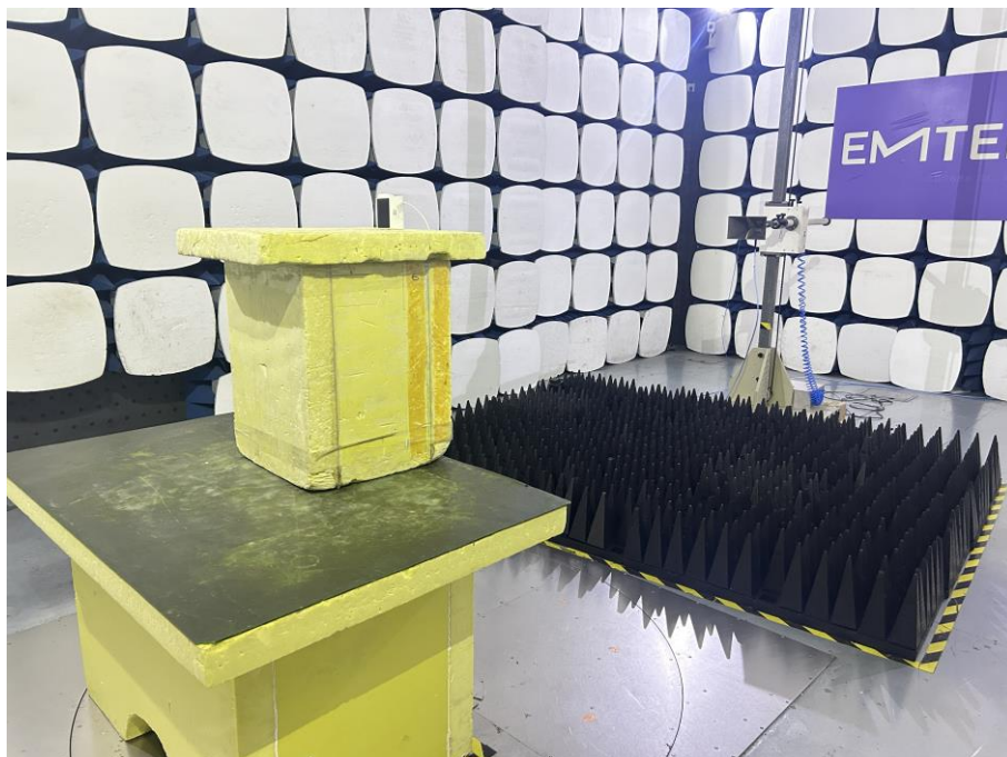
Spurious Emission Test Setup (Above 1GHz)
