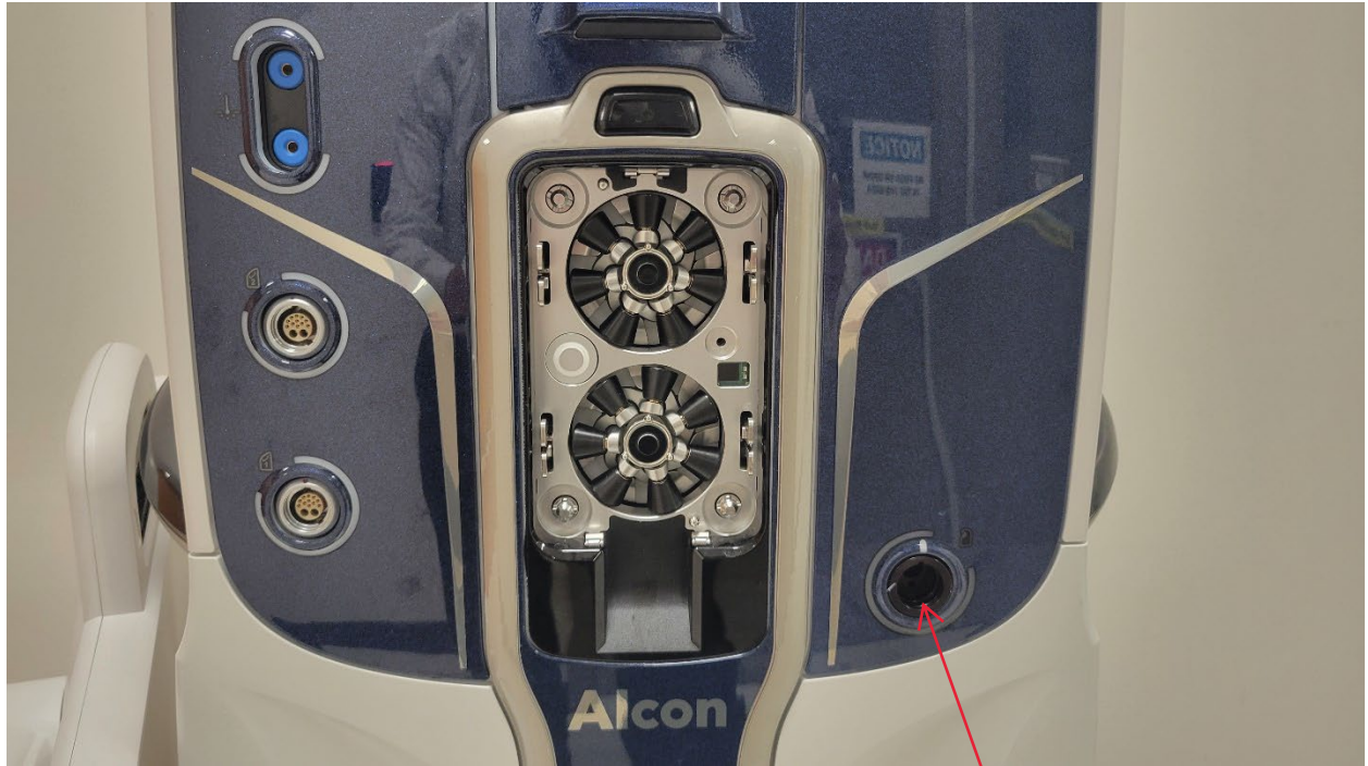
Unity CS front panel with RFID port
