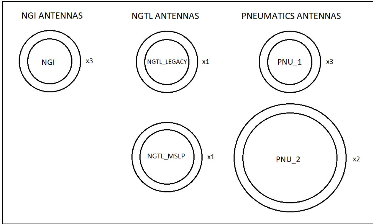
The NGI RFID PCBA (300038501) has three antennas, all identical in size (marked NGI above). The NGTL RFID PCBA (300035274) has two antennas, one smaller in size (marked NGTL\_LEGACY above) and one larger in size (marked NGTL\_MSLP above). The Pneumatics RFID PCBA (300036797) has five antennas, three smaller identical in size (marked PNU\_1 above) and two larger in size (marked PNU\_2 above).
