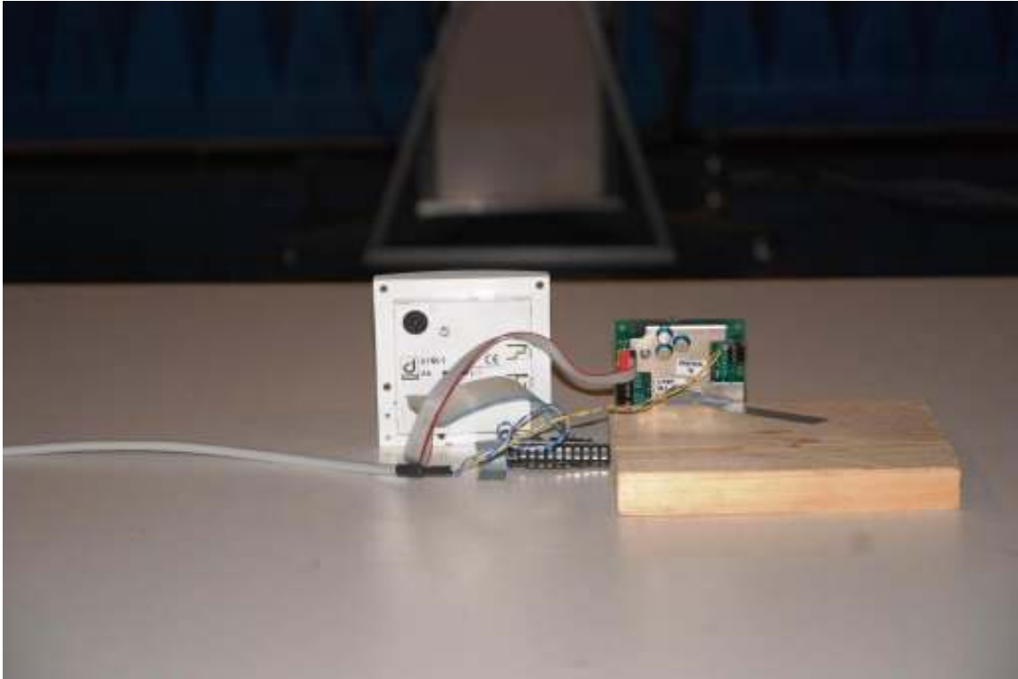
Fig. 6 Test setup rear side (30 MHz – 1 GHz)
