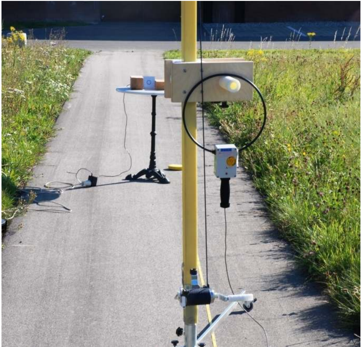
Fig. 4 Test setup (9 kHz – 30 MHz)
