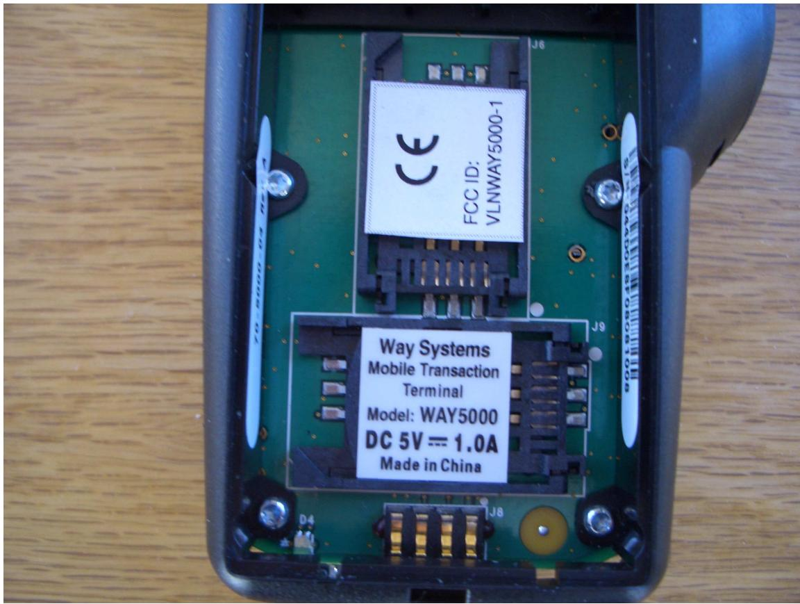
The picture above shows the four labels located in the battery compartment of the way5000. These labels are:
