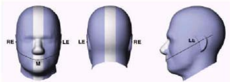
Figure 12.1 Front, back and side view of SAM Twin Phantom
