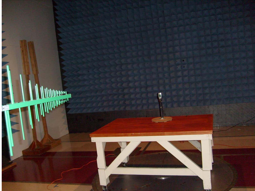
Photograph 2. Test Equipment and setup for various Radiated Measurements – Bilog Antenna
