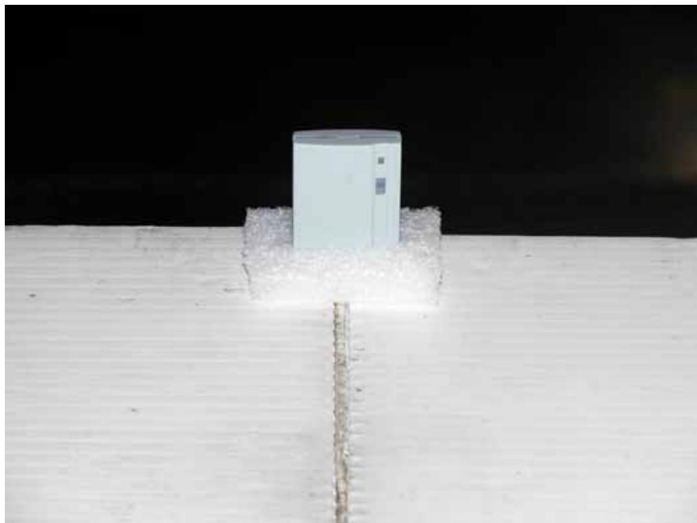
**RADIATED RF MEASUREMENT SETUP**
