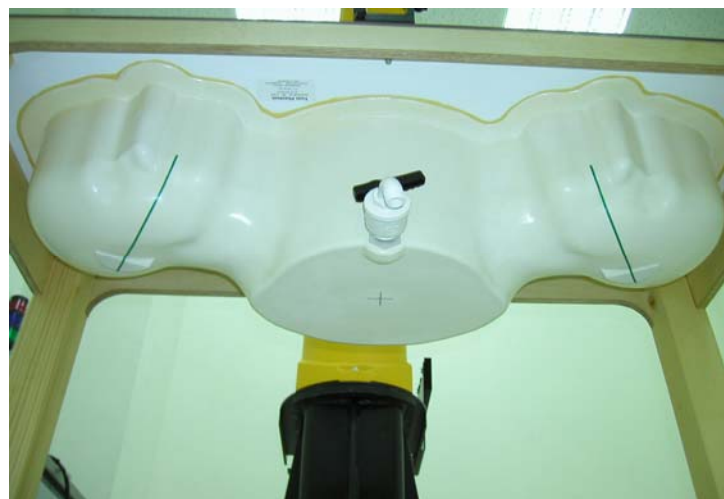
Fig. 5.4 Bottom view of twin phantom
