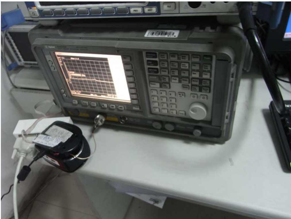
CONDUCTED TEST SETUP
