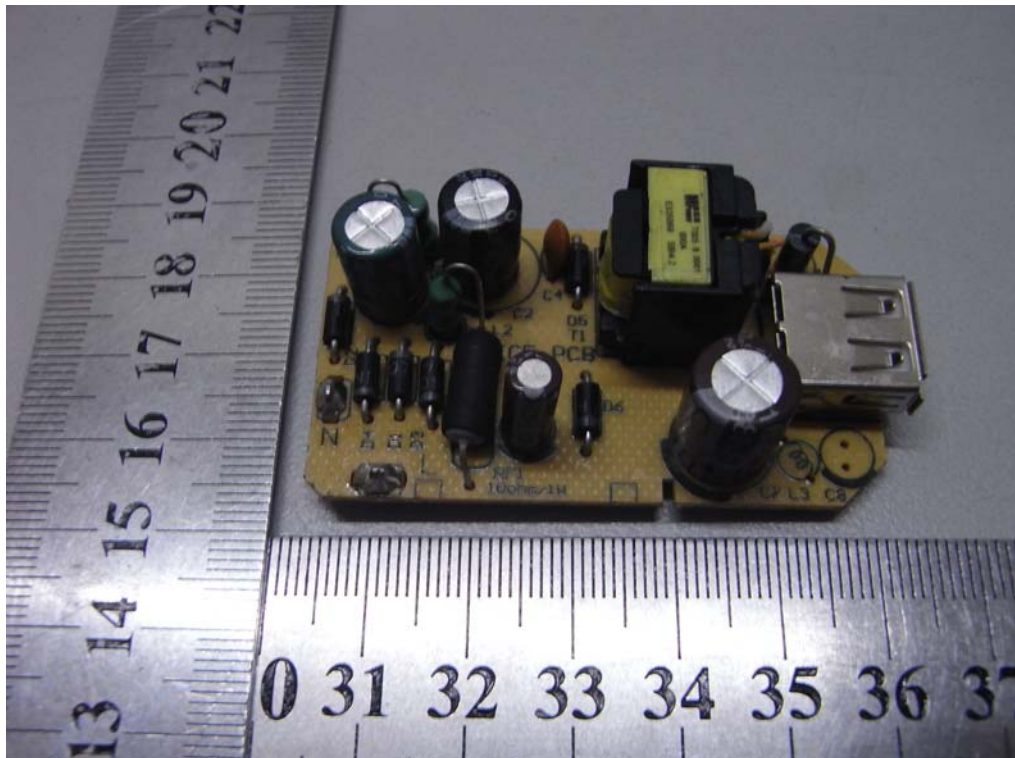
INTERNAL PHOTO OF AC/DC ADAPTER - Huoniu/HNB050070U
