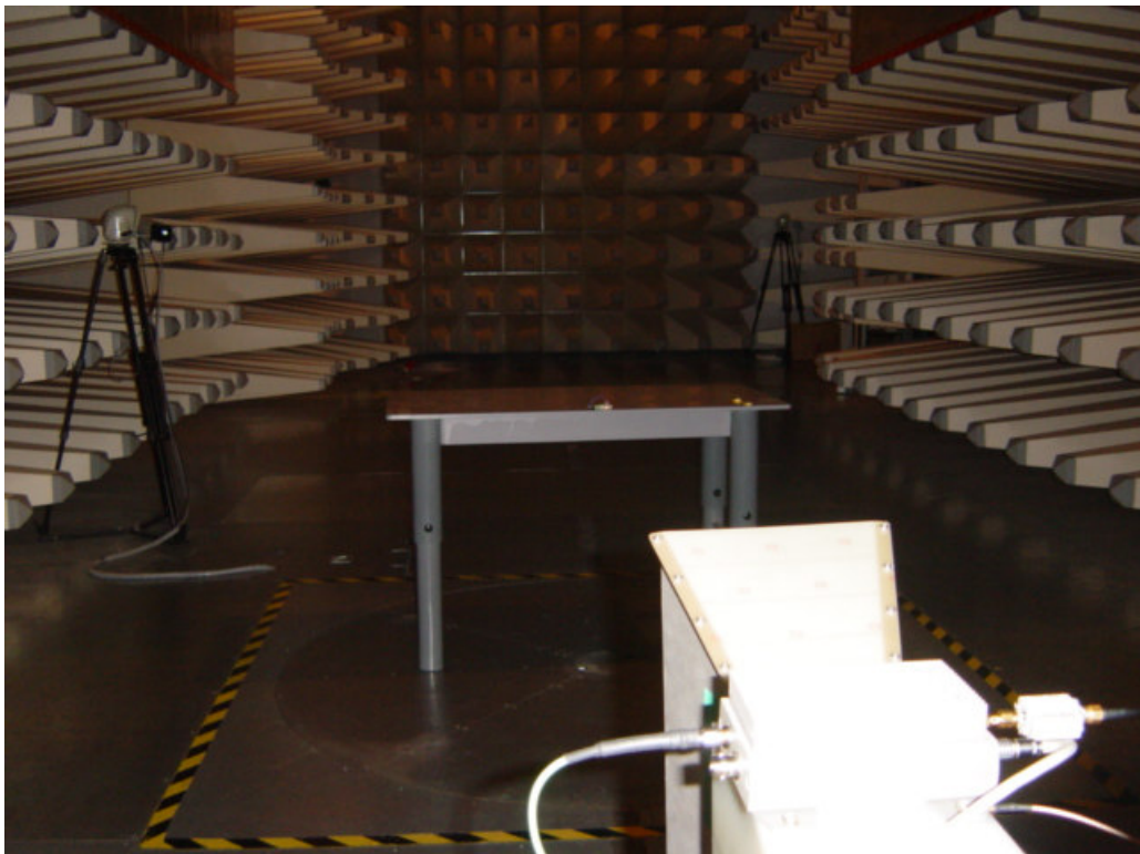
Set-up for Radiation Emission (Transceiver)
