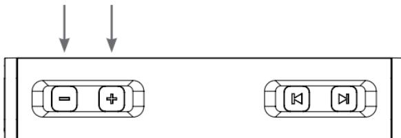
**TIP:** Because the volume control buttons of The Blaster do not control the volume output of your music device, you must properly adjust the volume settings of each device independently.
