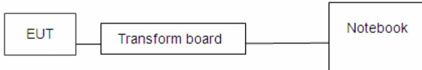
Note: 1. The EUT was programmed to be in continuously transmitting mode and the transmit duty cycle is not less than 98%.
