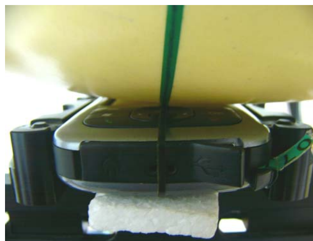
Fig.3 Right Head Section / Cheek-Touch Position
