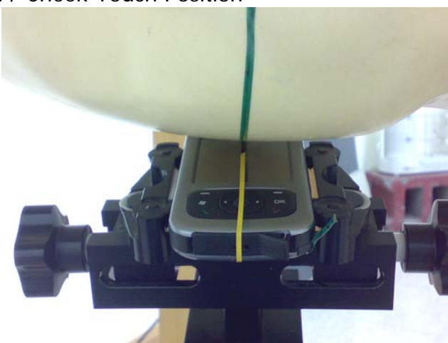
Fig.4 Right Head Section / Ear-Tilt Position(15°)
