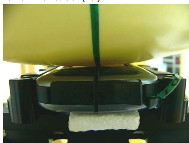
Fig.5 Left Head Section / Cheek-Touch Position
