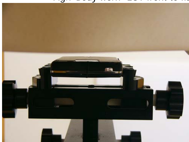
Fig.8 Body worn- EUT back to flat phantom (testing in GPRS Mode)
