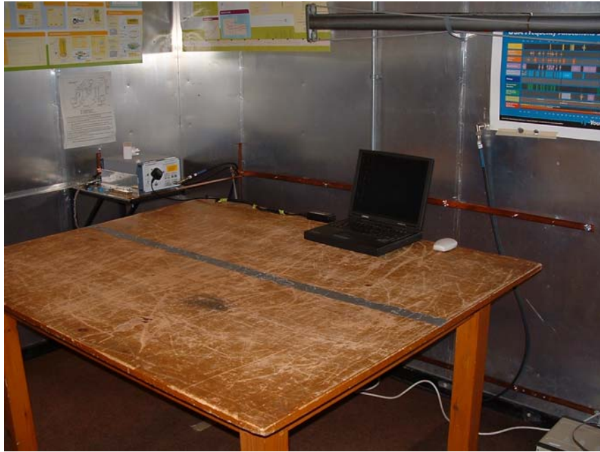
Test Setup Powerline Conduction
