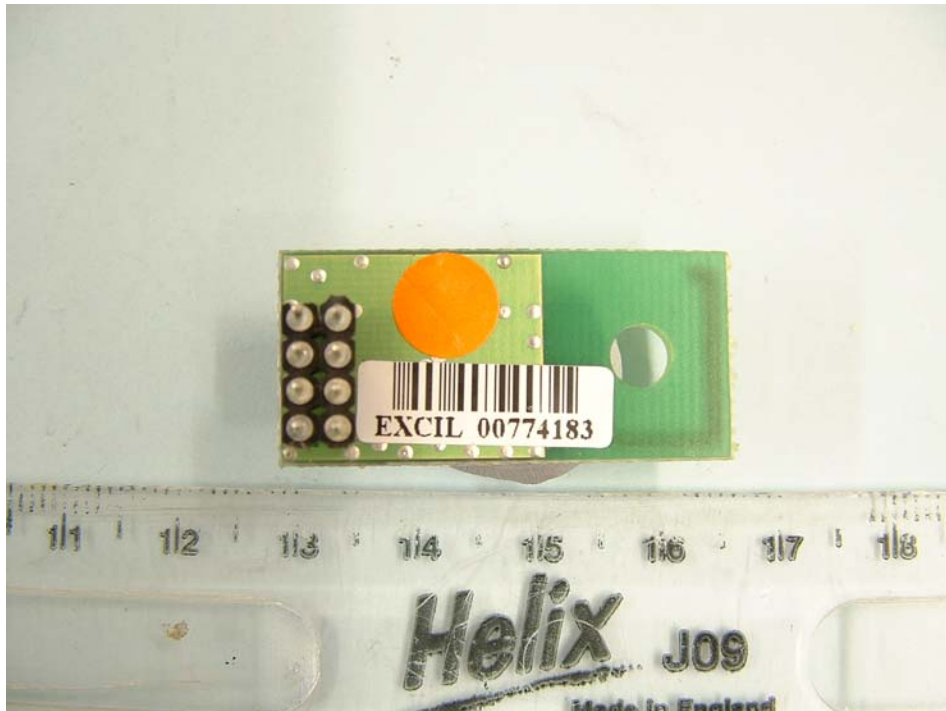
Radio Module Track Side
