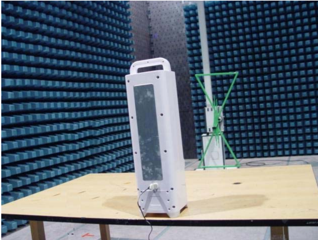
Photo 3 Radiated Emission Test
