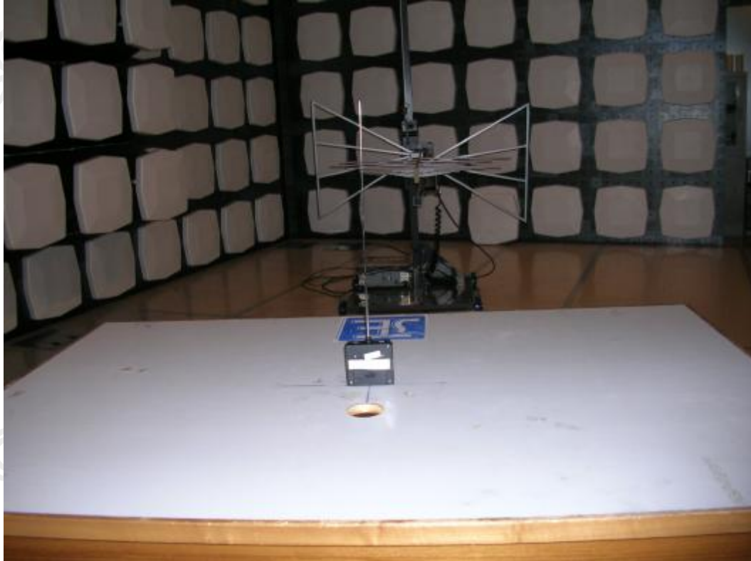
Measurement of Radiated Emission Test Set Up
