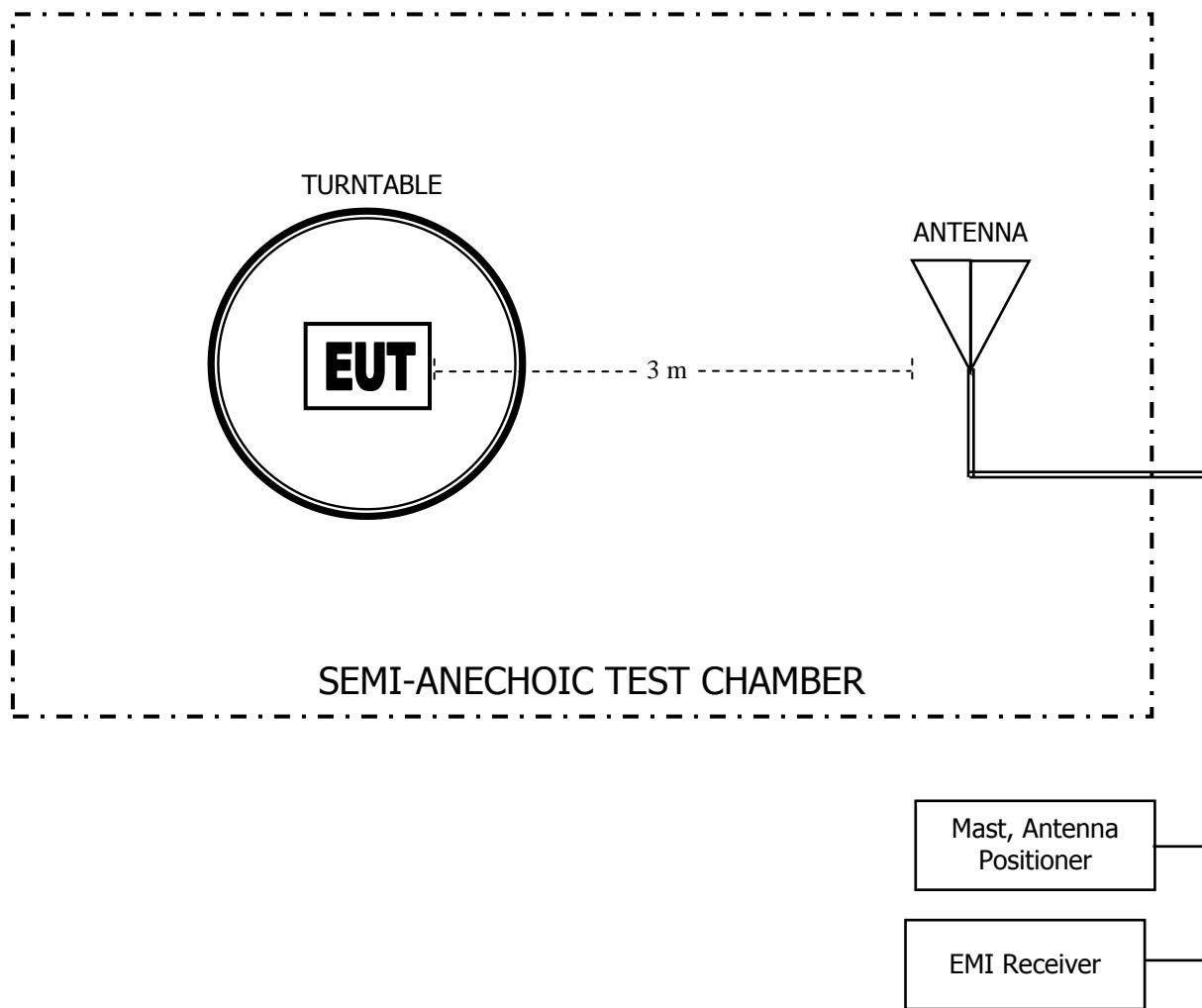
**FIGURE 3: RADIATED EMISSIONS 3-METER
