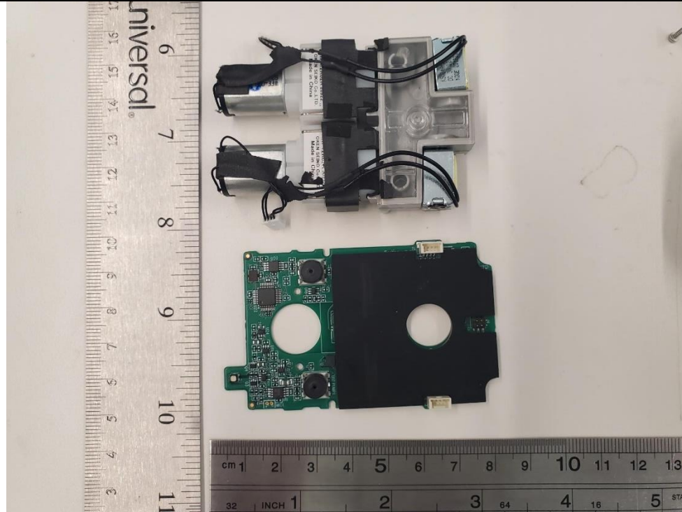
Back view of p/n: 27781 (Griffon NiBP V3 Circuit Board Assembly) with assembly, Wire Harness, Griffon Pump + Valve
