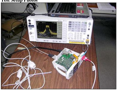
Test Conditions: The EUT is on the table and all the probes and cables are connected to the unit. Measurements are made by direct connect with the Serial cable connected to the laptop computer, which is used to change the TX characteristics. The 32db offset is 20 db for the attenuator, 2 db for the antenna gain. The other 10 db is the bandwidth integration.
