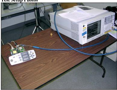
**Test Conditions:** The EUT is on the table and all the probes and cables are connected to the unit. Measurements are made by direct connect with the Serial cable connected to the laptop computer, which is used to change the TX characteristics. There is a 1.4 dB offset to correct for the cable.
