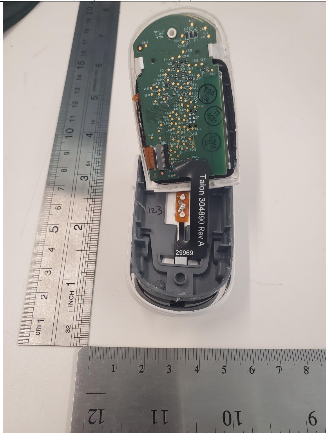
Internal view after opening the front cover with display to show back side of board 29911
