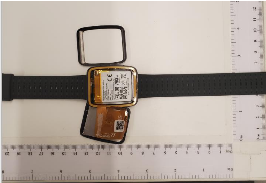
Photo 1: Internal top view of W1 displaying battery and LCD back side
