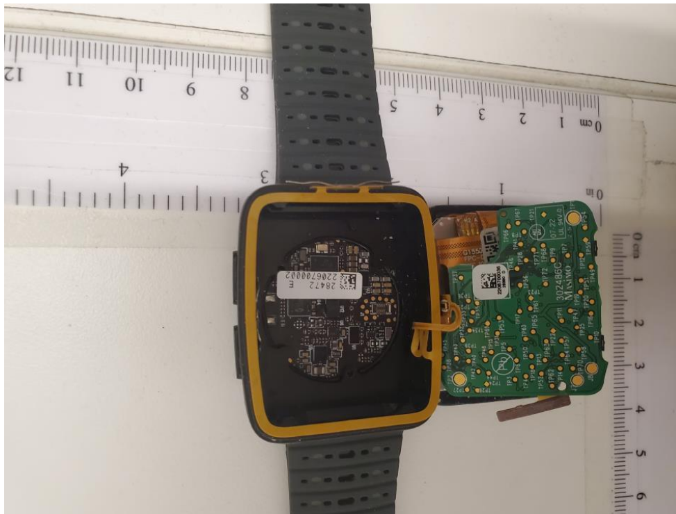
Photo 6: Close up view on bottom PCB
