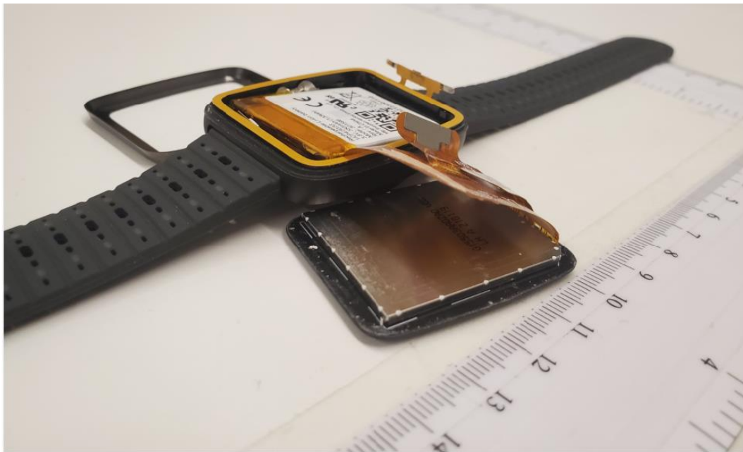
Photo 2: Internal right view of W1 displaying battery and LCD back side, another view
