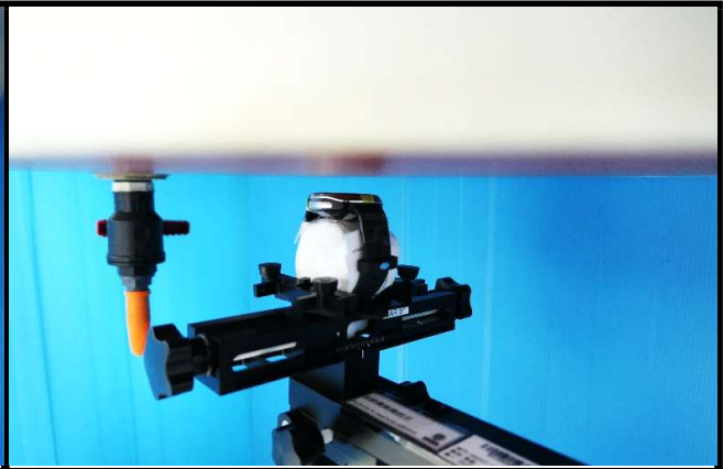
Front Face of EUT Tested at 10 mm for NFC
