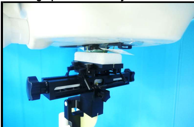
Rear Face of EUT Tested at 0 mm for WWAN / WLAN / BT
