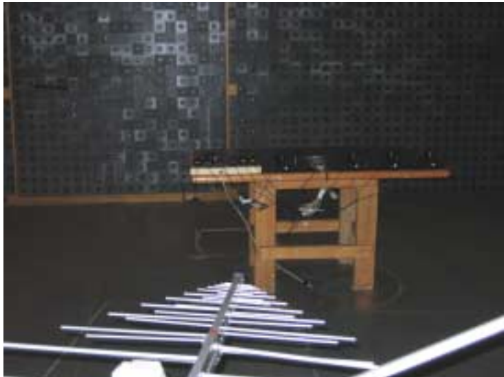
Photograph No.6 Setup for radiated emission measurements in the anechoic chamber
