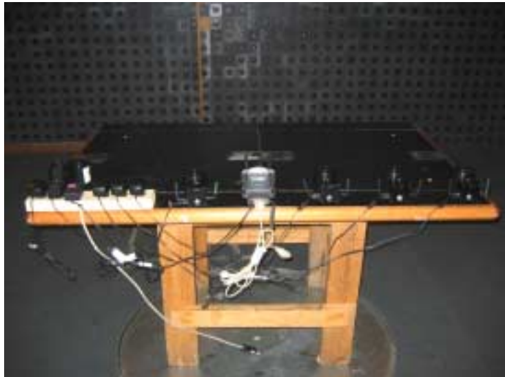
Photograph No.7 Setup for radiated emission measurements in the anechoic chamber
