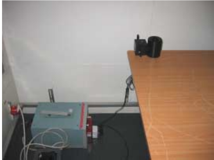
Photograph No.5 Setup for conducted emission measurements on the EUT power ports
