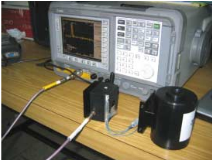
Photograph No.1 Setup for peak output power, peak spectral power density, OBW and spurious emission measurements
