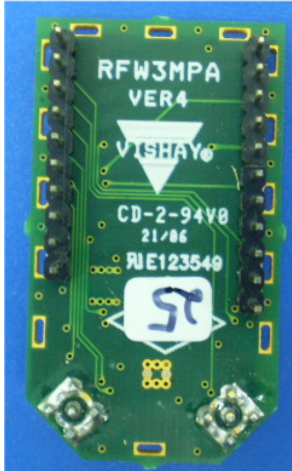
Photograph No.6 Print side of the RF PCB
