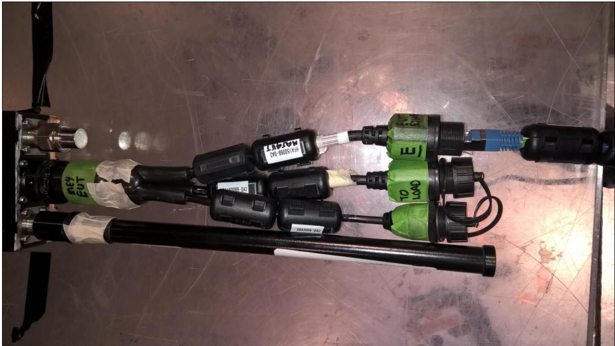
Photograph 3. Radiated Emissions Below 1 GHz, Modification to Support Equipment 3
