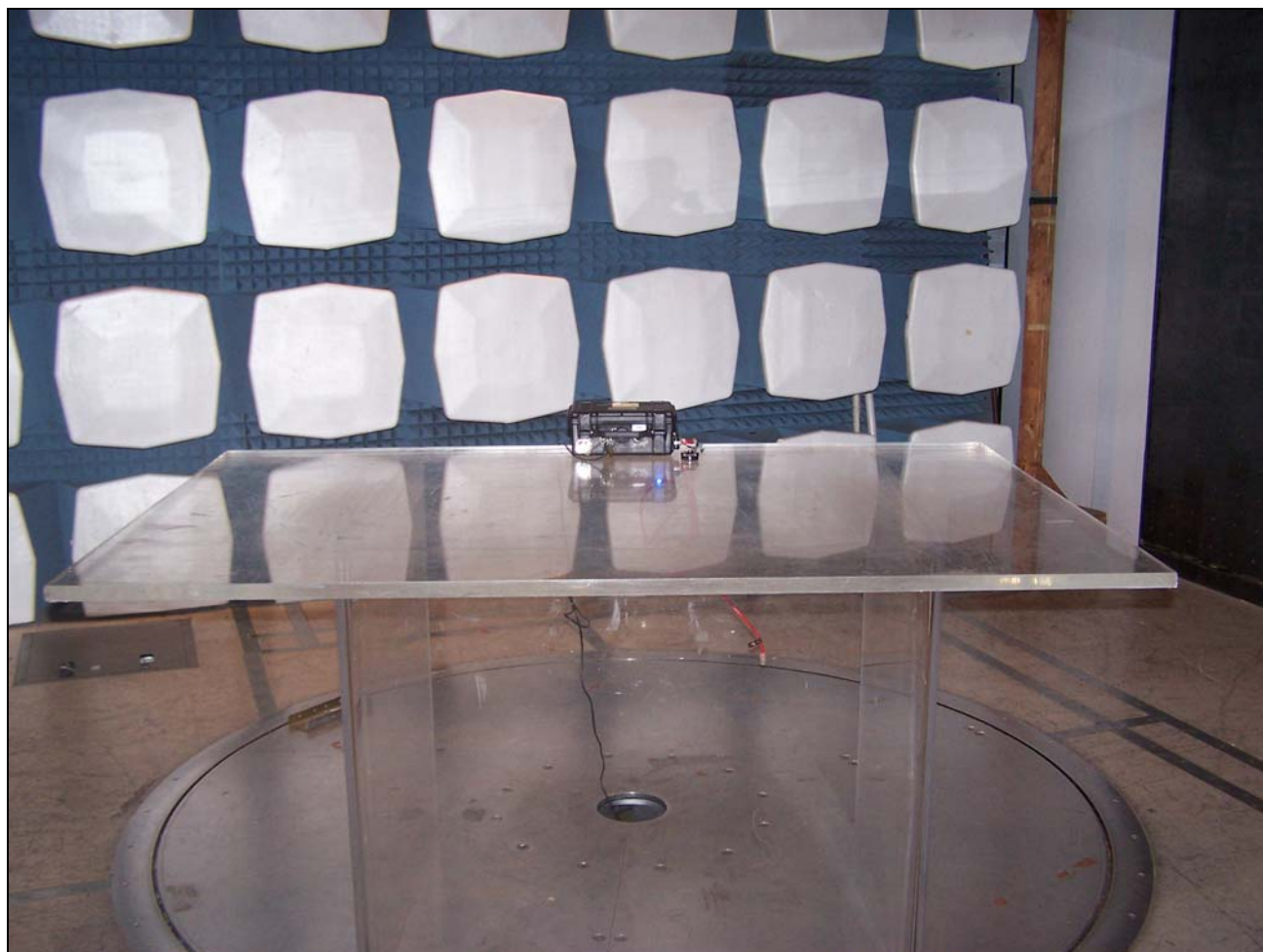
Photograph 2. Radiated Emissions Test Setup
