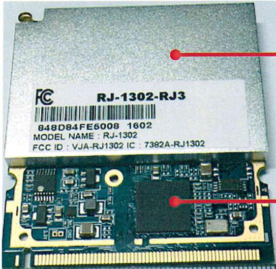
Critical RF components such as High Power PA for TX Path and LNA for RX path are housed below this RF shielding
