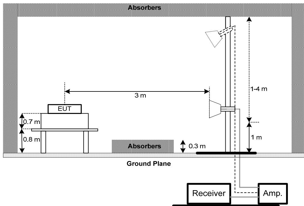
(C) For radiated emissions below 30MHz
