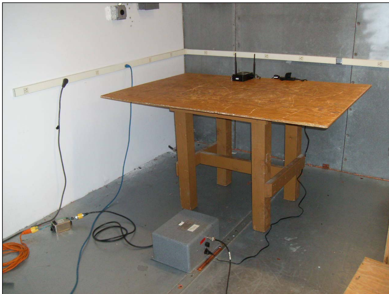
Photograph 4. Conducted Emissions Test Setup
