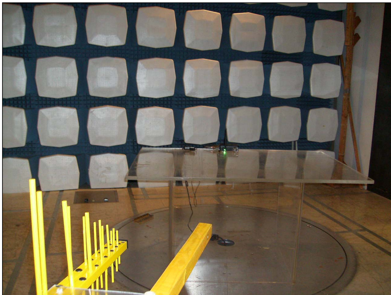
Photograph 5. Radiated Emission Limits Test Setup
