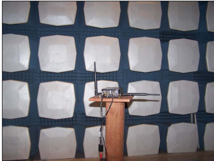
Photograph 2. Spurious Radiated Emissions, Test Setup
