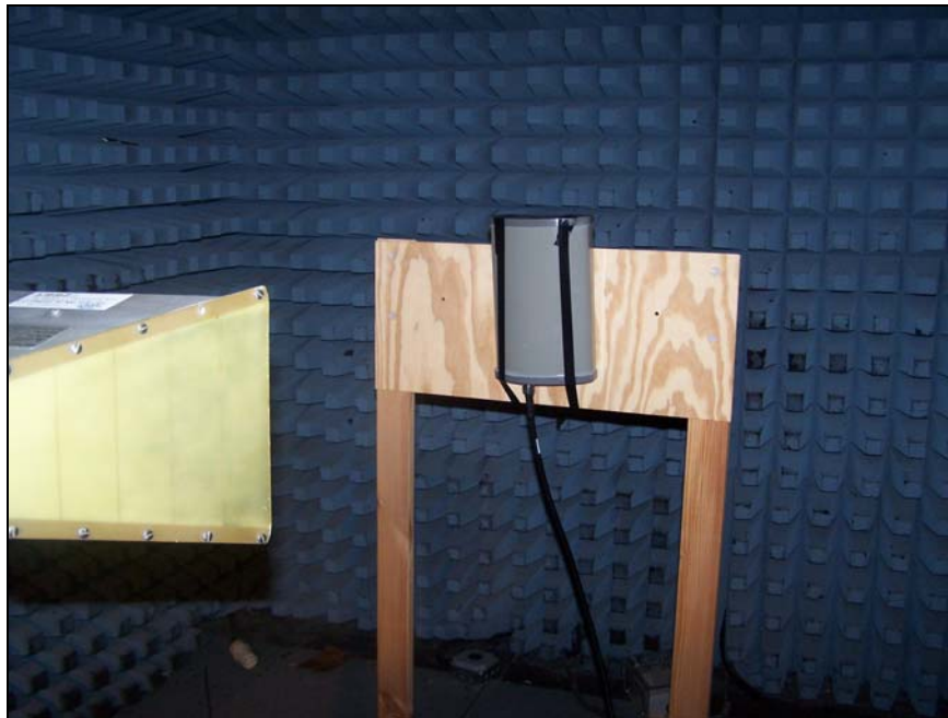
Photograph 4. Spurious Radiated Emissions, Test Setup, 120 deg 9 dBi sector Antenna
