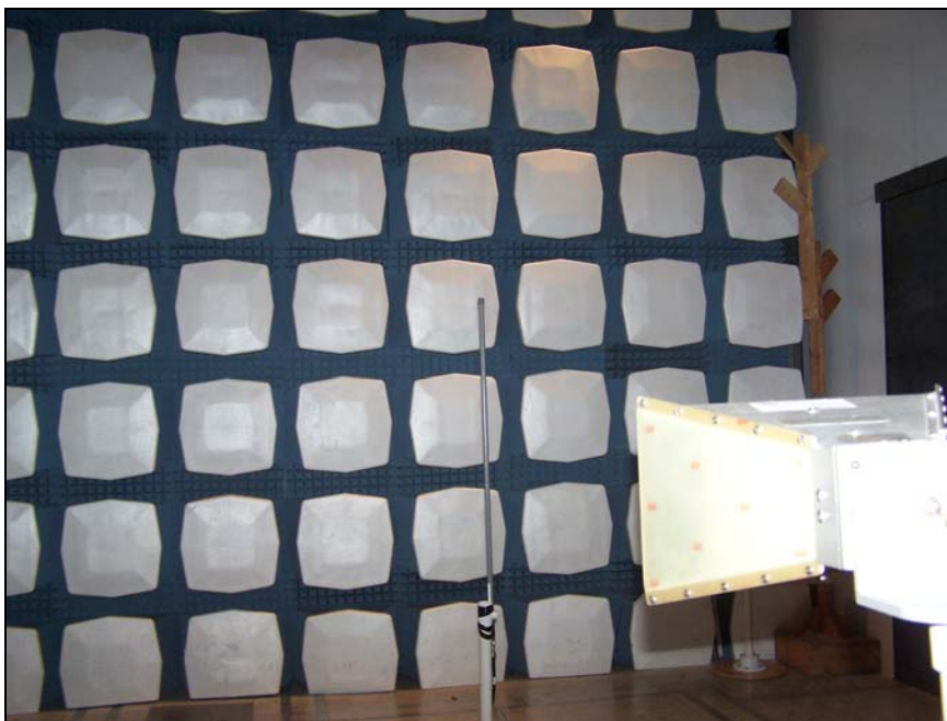
Photograph 1. Band Edge Emissions, Test Setup
