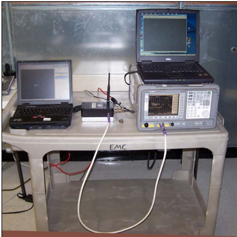
Photograph 3. 6 dB Bandwidth Test Setup
