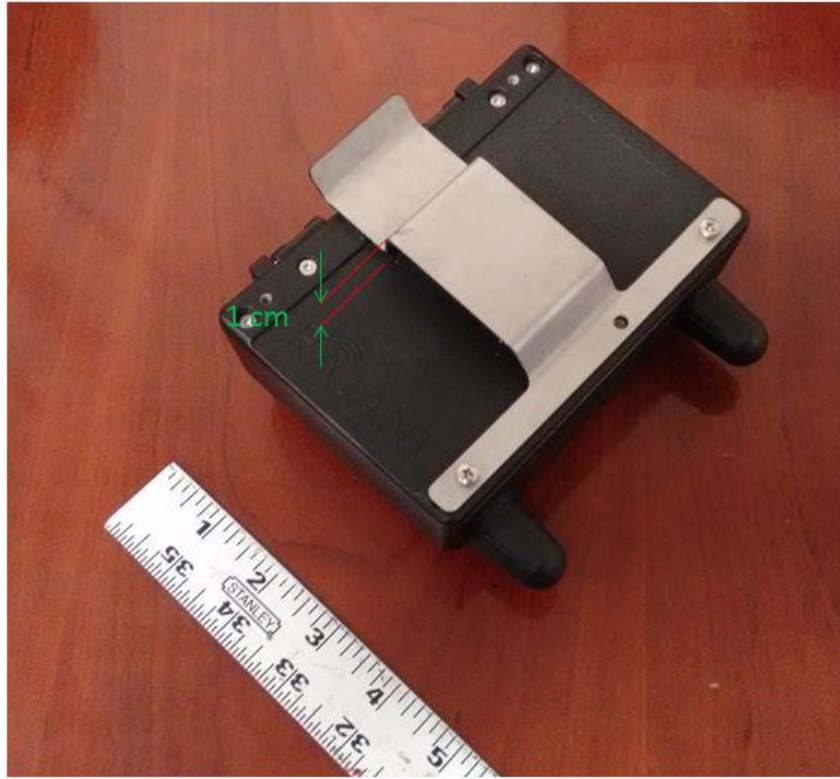
Figure 25. EUT with belt clip separation illustrated
