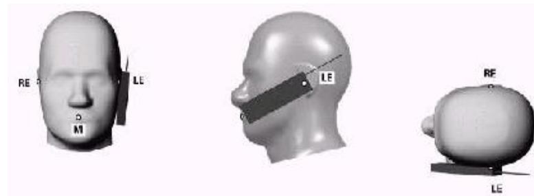
Figure 9. Front, Side and Top View of Cheek/Touch Position
