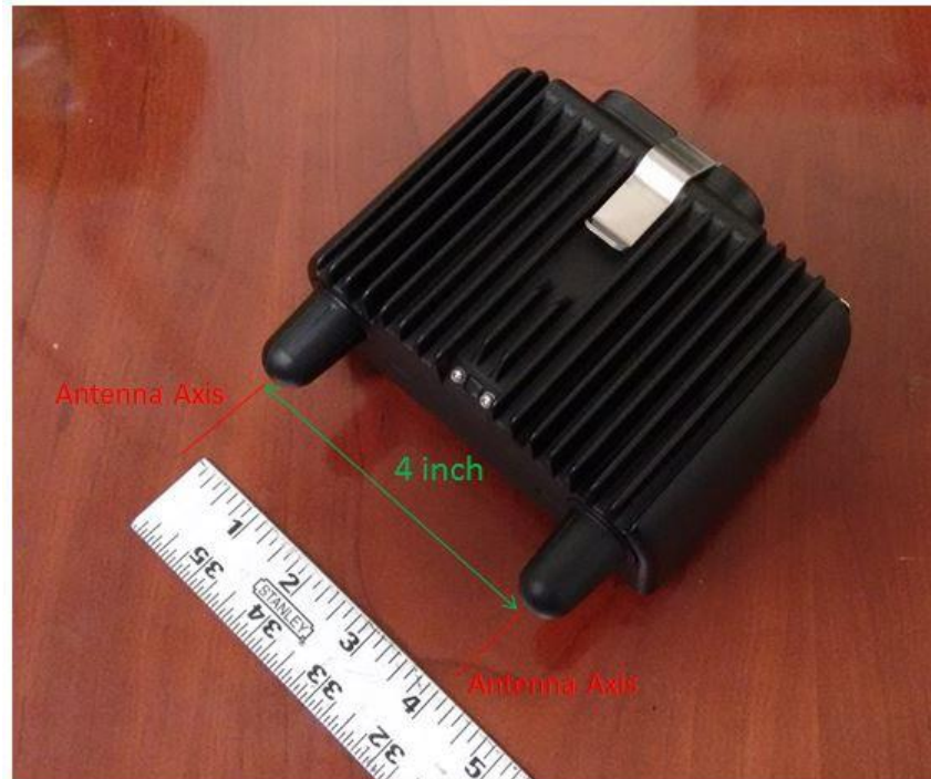
Figure 4. Rajant CX1-3600 with antenna separation illustrated
