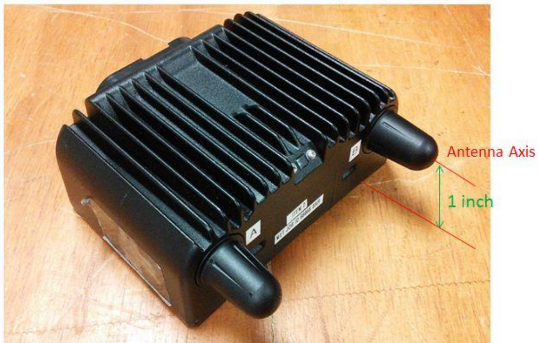
Figure 5. Rajant CX1-3600 with antenna separation illustrated
