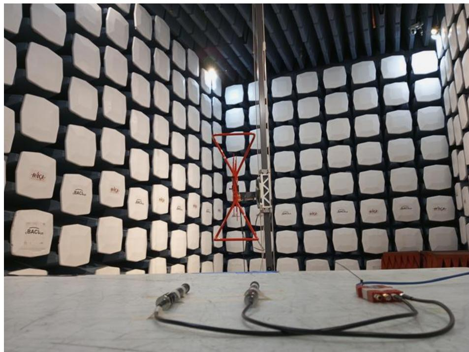
**1.5 WLAN0 Radiated Spurious Emissions: 1-18 GHz at 1 meter**5.0-7.2 GHz Omnidirectional Antenna (PUCK-12)
