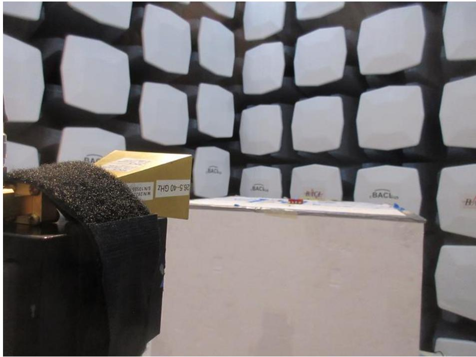
**1.14 WLAN1 Radiated Spurious Emissions: 26.5-40 GHz Rear View at 1 meter**
