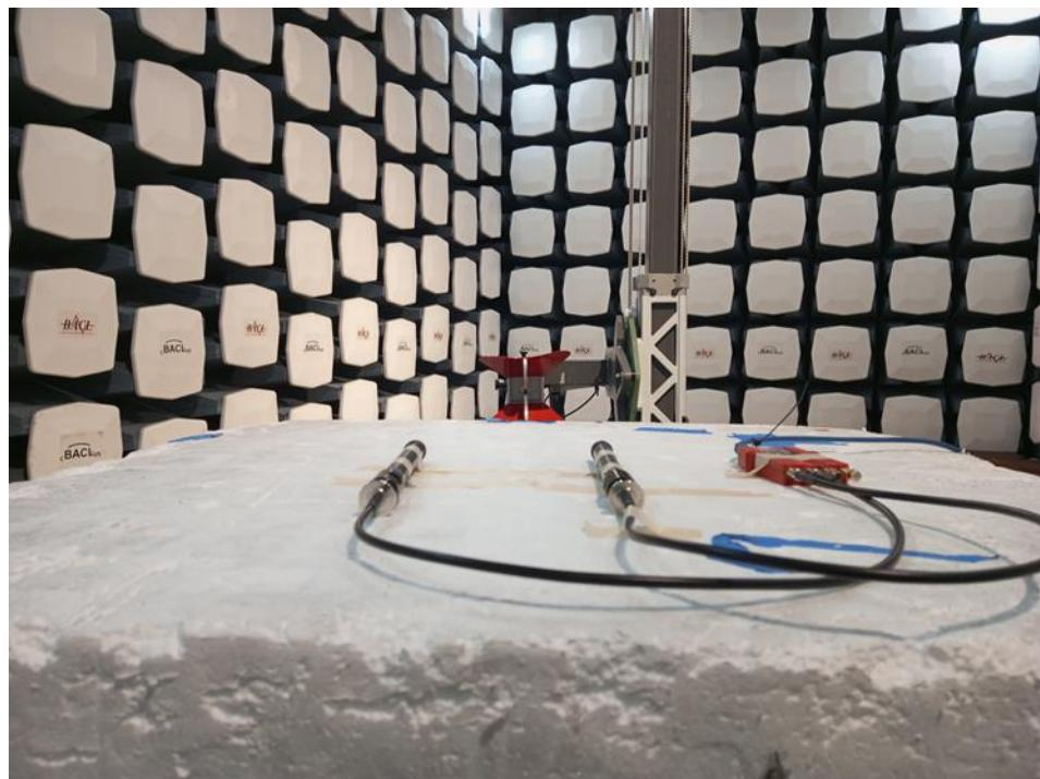
**1.6 WLAN1 Radiated Spurious Emissions: 1-18 GHz at 1 meter****5.0-7.2 GHz Omnidirectional Antenna (PUCK-12)**
