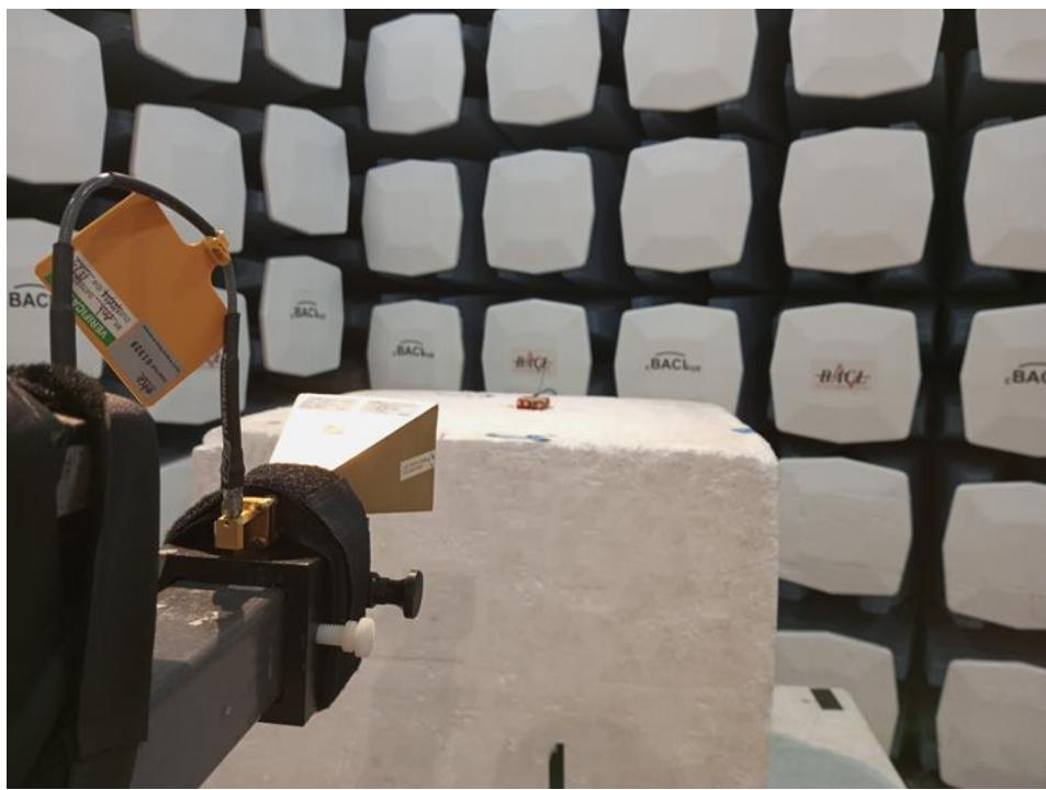
**1.8 WLAN0 Radiated Spurious Emissions: 18-26.5 GHz Rear View at 1 meter**
