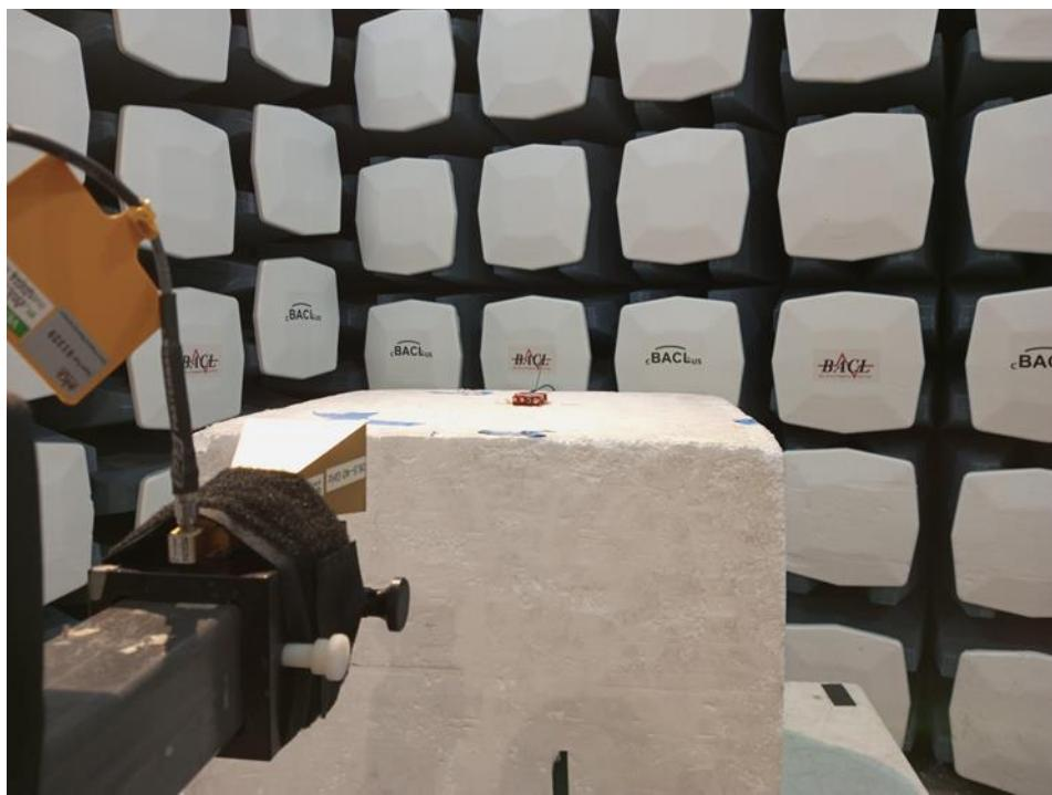
**1.12 WLAN0 Radiated Spurious Emissions: 26.5-40 GHz Rear View at 1 meter**
