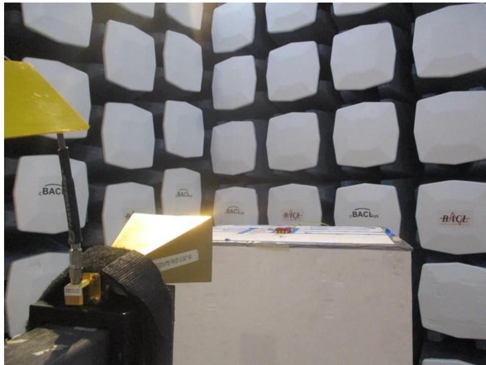
**1.10 WLAN1 Radiated Spurious Emissions: 18-26.5 GHz Rear View at 1 meter**
