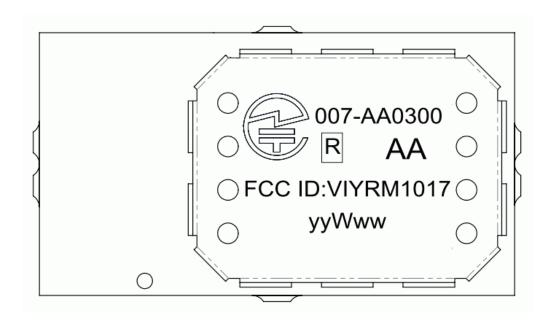
FCC ID will be displayed on the shield case by laser marking.
