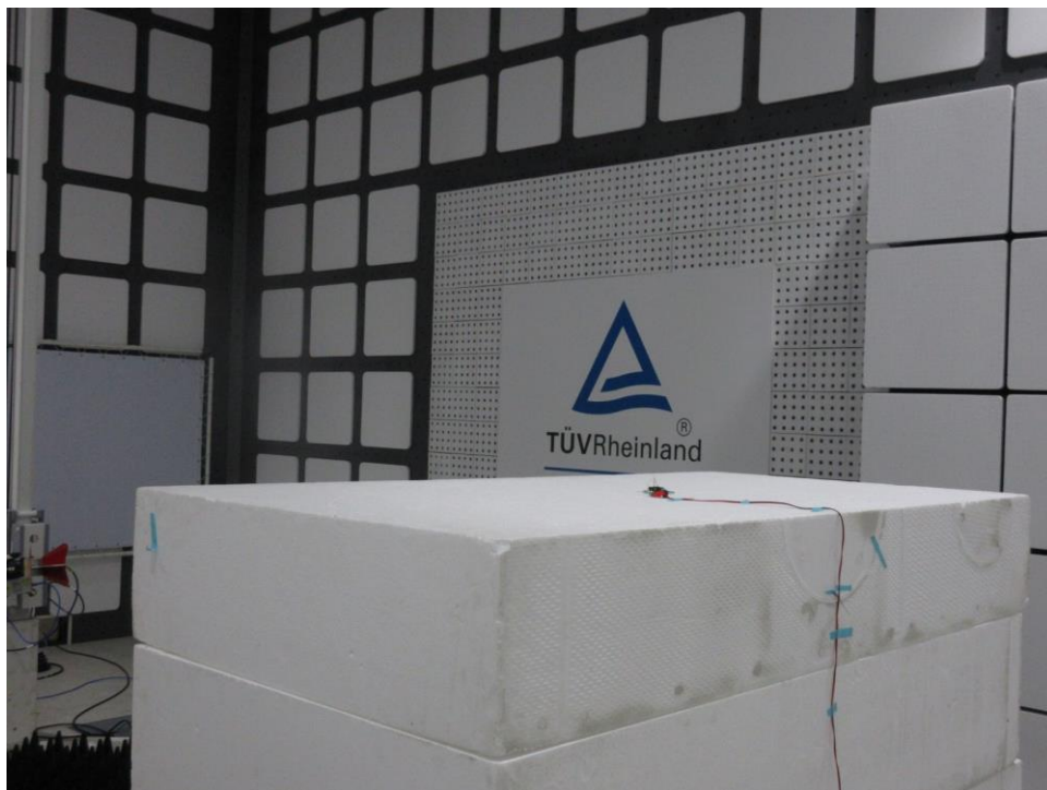
Photograph 2: Set-up for Spurious Emissions (Front View 2)
