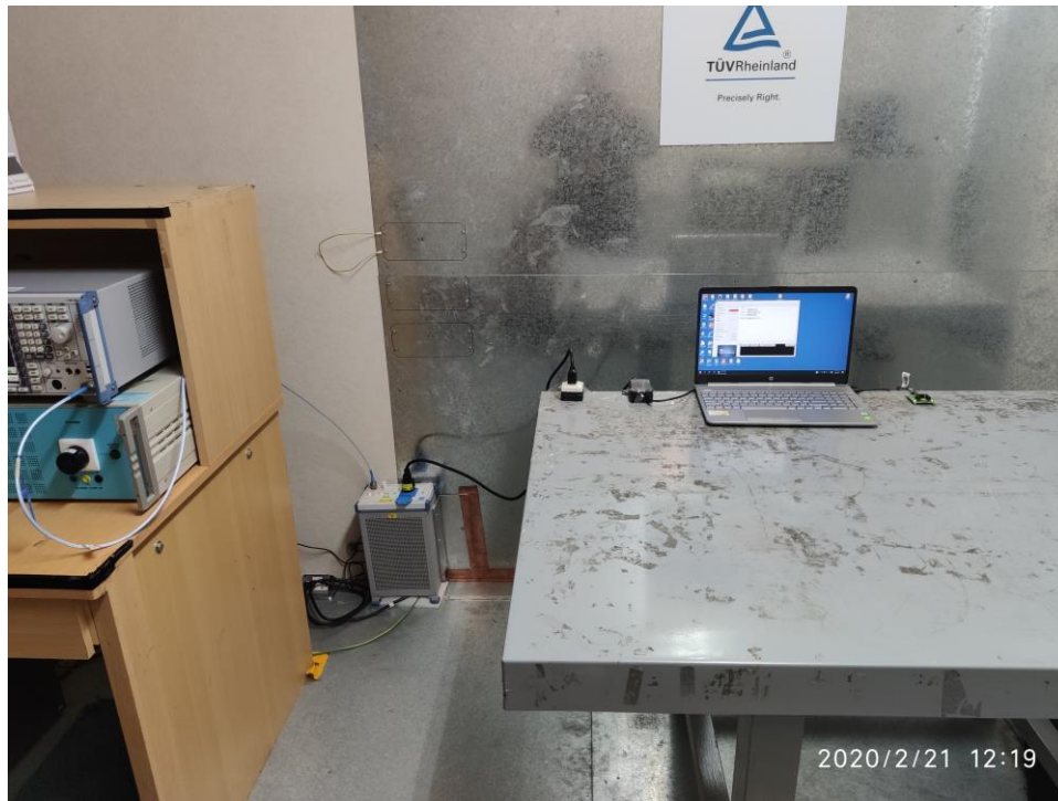
Photograph 8: Set-up for Mains Conducted testing (Back View)
