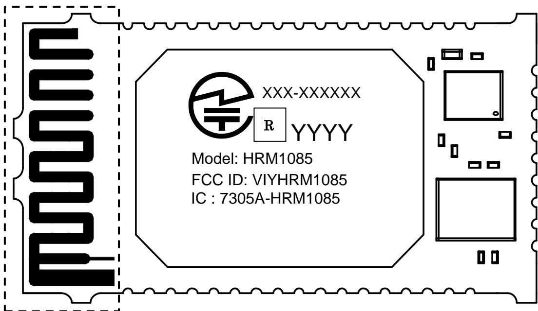
The label is printed with a laser on a shield case.
