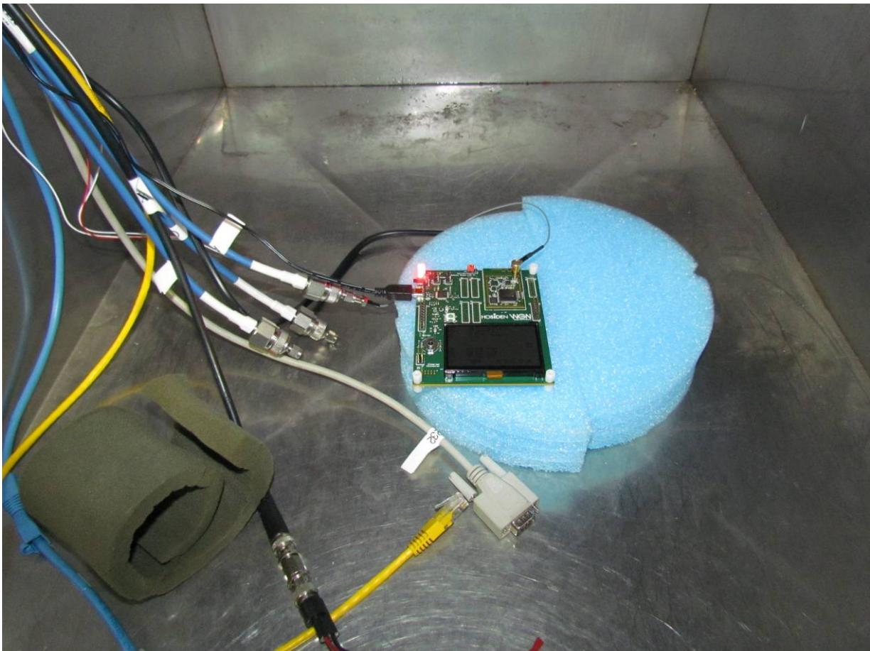
Transmitter Radiated Spurious Emission above 1 GHz
