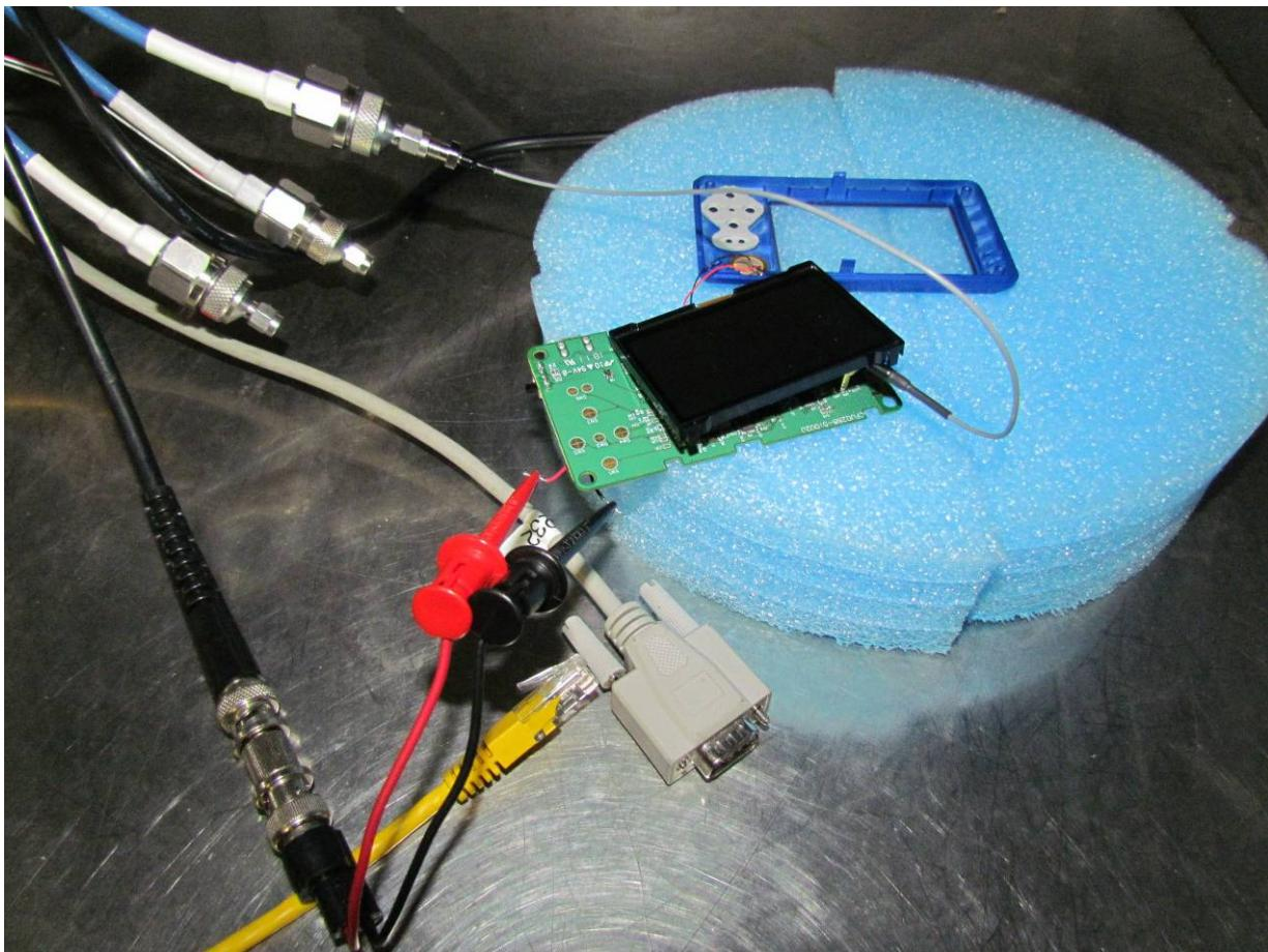
Transmitter Radiated Spurious Emission above 1 GHz
