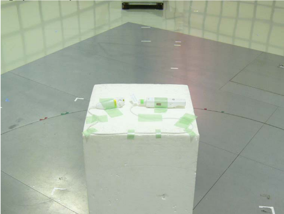
Photograph 9: Set-up for Radiated Emission of Receiver, Front View
