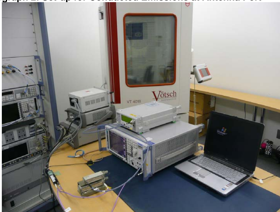
Photograph 2: Set-up for Conducted Emissions at Antenna Port
