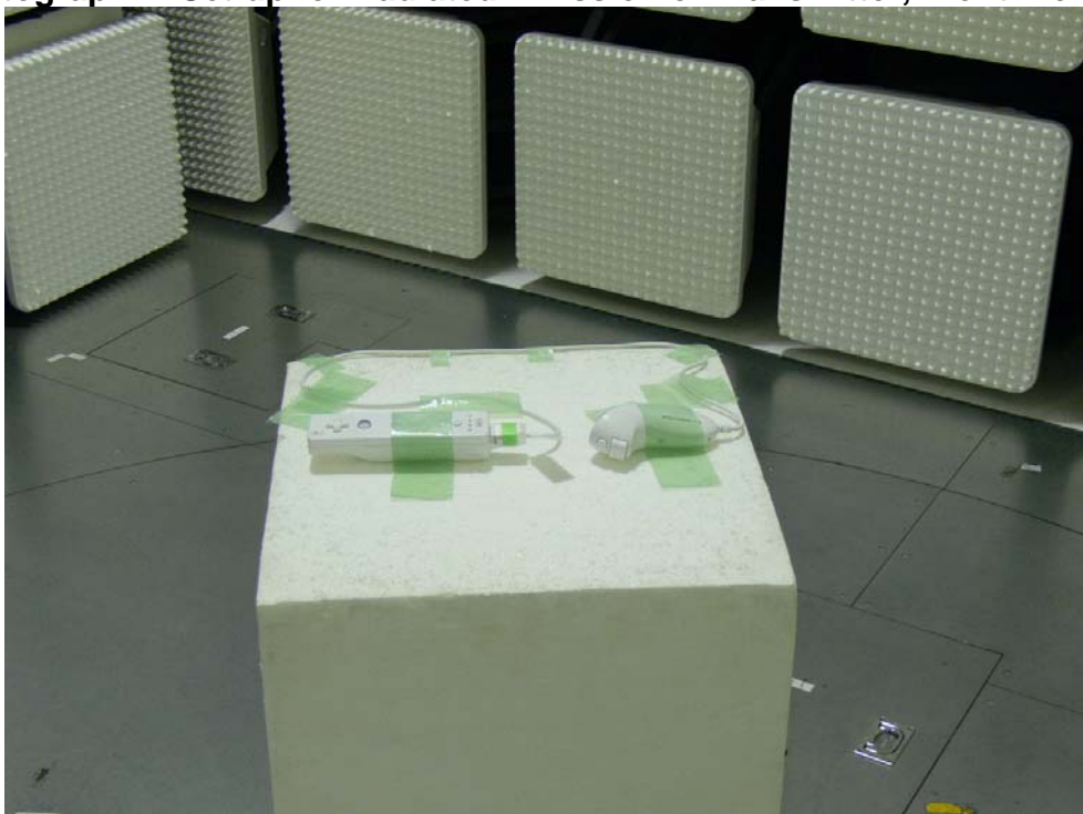
Photograph 7: Set-up for Radiated Emission of Transmitter, Front View
