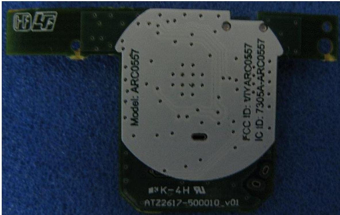
Following IDs are displayed on backside of PWB with silk printing.
