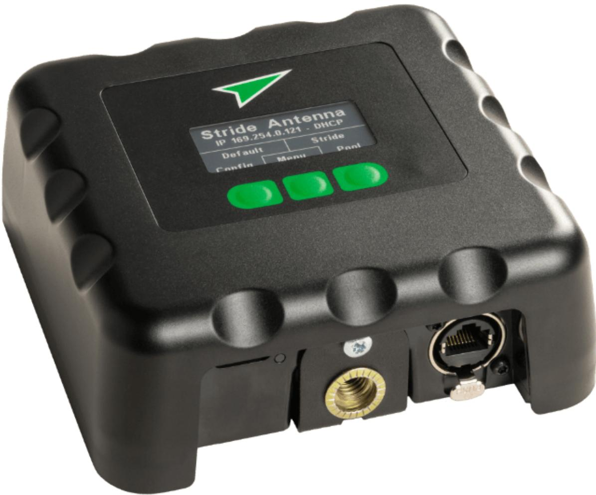
The Green-GO STRIDE DECT Antenna introduces next-generation wireless intercom capabilities through synchronized multi-antenna coverage and seamless roaming. Operating via PTPv2 network synchronization, the system eliminates traditional handover gaps from the past while accommodating up to five simultaneous client connections per antenna.
