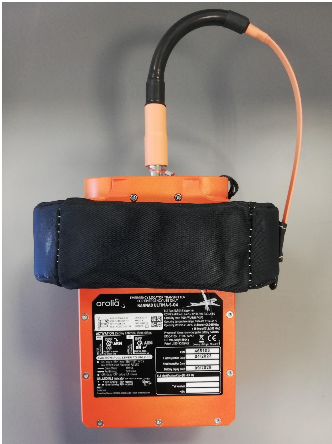
Figure 7 beacon with floating collar
