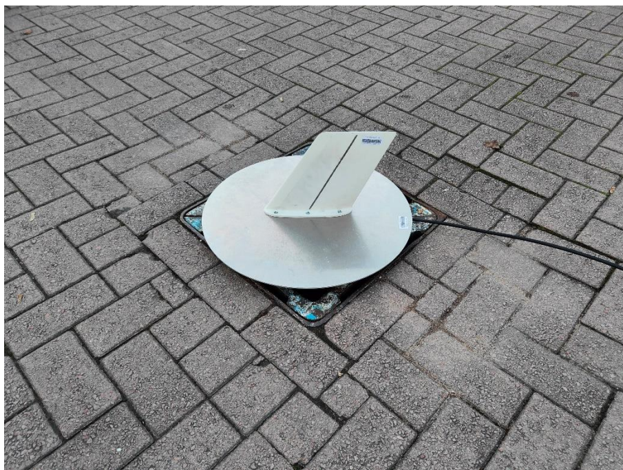
Figure 5 - Radiating Antenna Position for Satellite Qualitative Setup
